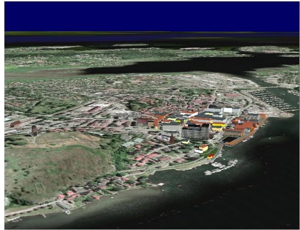
Figure 2. 3D Model from Toensberg with textured terrain and additional building objects of the city. In the background lower resolution parts are visible (view from the TellMarisOnBoard application).
